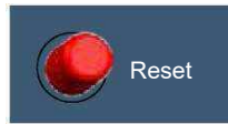
When the intelligent controller is in the protection state, the circuit breaker is open. After clearing the line fault, press this button to close the circuit breaker.
