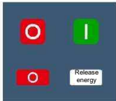
Circuit breaker being open without stored energy
