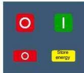
Circuit breaker being open with stored energy
