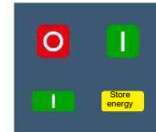
Circuit breaker being closed with stored energy
