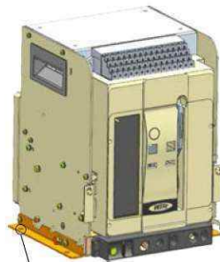
External installation position of the drawer mode circuit breaker
