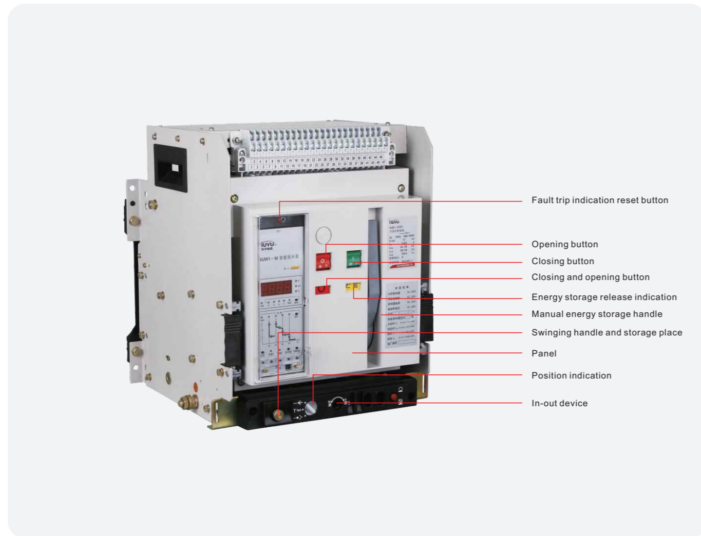
Fig.5 HUW1PVA,HUW1F ACB operating indicator diagram
