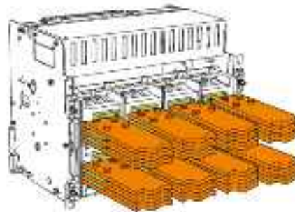
Horizontal wiring mode of 1,600 A and above
